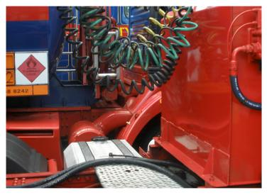
Drivers working outside the vehicle are exposed to slipping and tripping dangers every time they cross the catwalk behind the cab or walk across a trailer bed.
